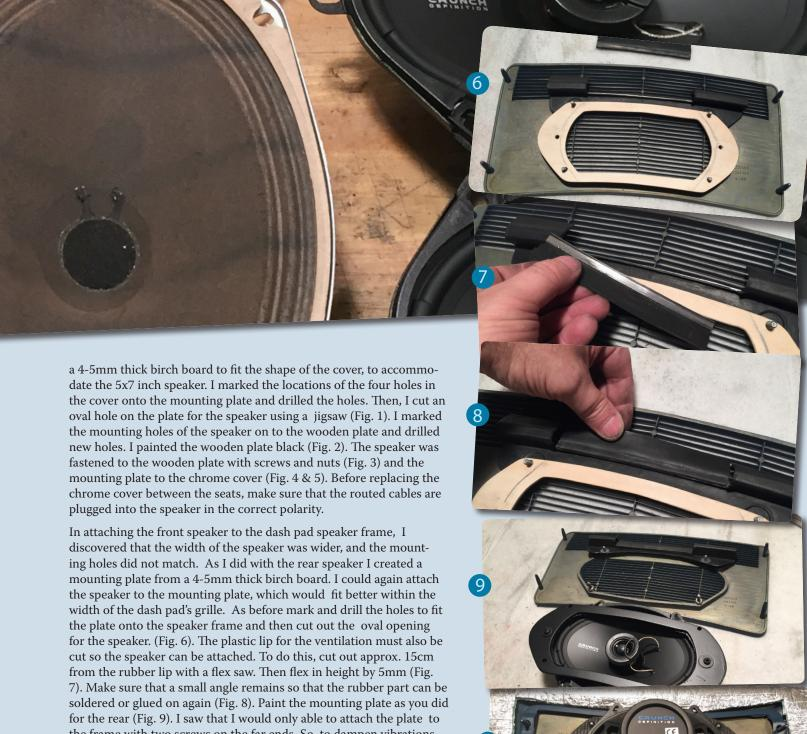
the frame with two screws on the far ends. So, to dampen vibrations I glued a thin rubber mat between the speaker and the plate before I attached the plate to the frame (Fig. 10). Before attaching the frame to the dash pad pay attention to polarity! (Fig. 11)
